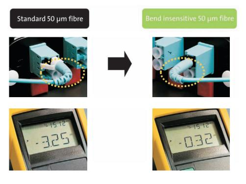
A single tight bend can cause a signal loss of over 3 dB, that's a 50% power reduction: such power loss would cause a 10 G link to fail! A bend insensitive multimode fibre under the same condition will exhibit 10 times less loss and so maintain a strong signal and no link failure.
