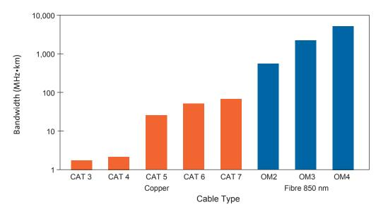
Bandwidth comparison of copper\* and fibre\*\* cables. OM2 fibre bandwidth capability has outlived all generations of copper cable design; OM3 and OM4 bandwidth and link length capabilities are even further beyond that of copper. \*Bandwidth frequencies for copper are typically referenced to 100m, here they are normalised to 1km. \*\*Fibre bandwidth refers to laser bandwidth at 850nm (Source: ISO/IEC 11801)
