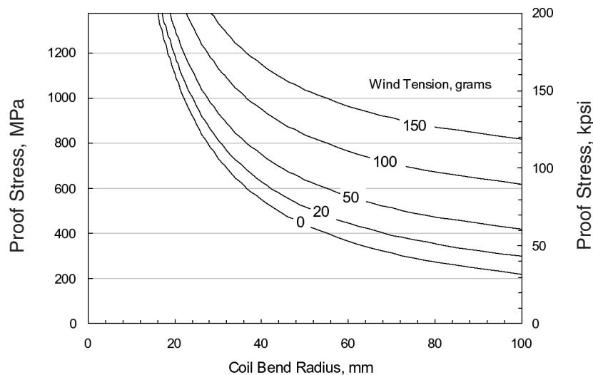
**Figure 1.** Proof test design diagram for optical fiber permanently wound on bobbins.
