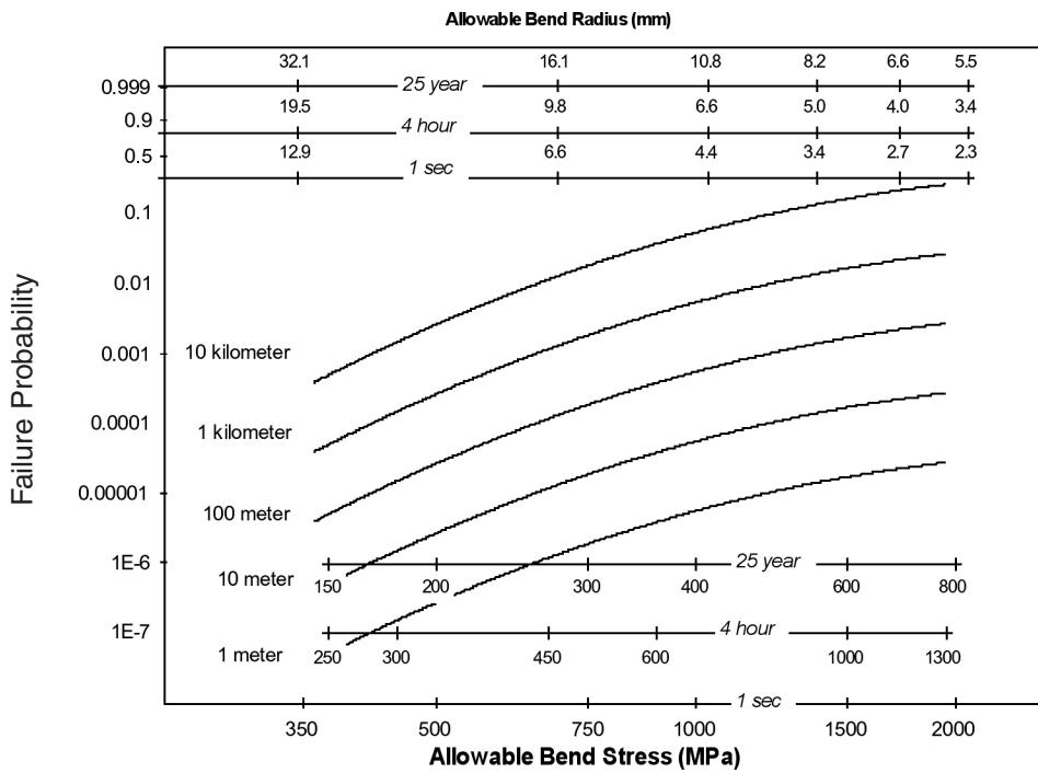
**Figure 3.** Design diagram for standard single-mode optical fiber in bending.
