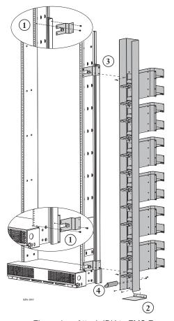
Figure 1 — Attach IBU to FMS Frame
