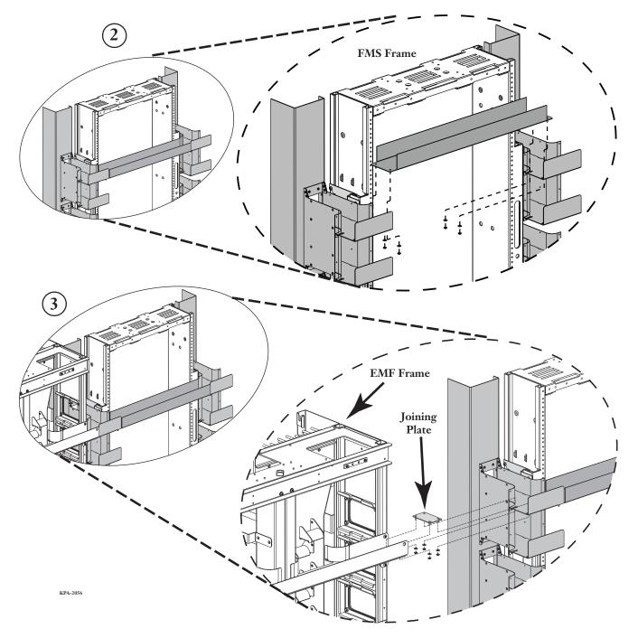
Figure 2 — Double IBU with Trough Connections
