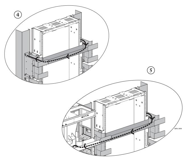
Figure 4 — Route Jumpers through the Trough
