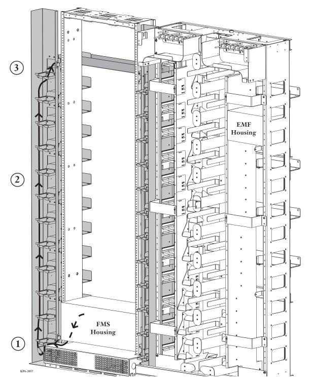
Figure 3 — Fiber Routing
