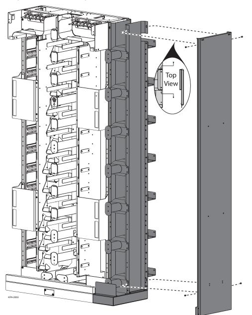
Figure 10 — Installing End Guard
