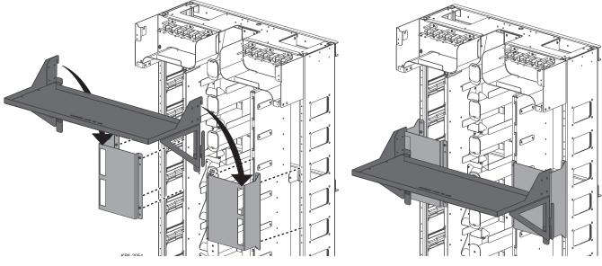
Figure 4 — Using Workshelf without Housing in Frame
