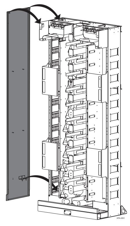
Figure 8 — Installing Endcap
