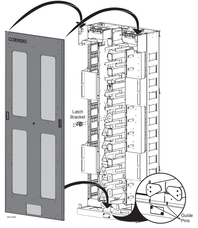
Figure 7 — Installing Single Door
