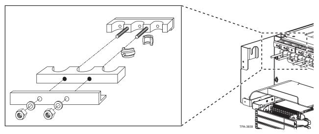
Figure 2 — Remove Existing Strain-relief Components
