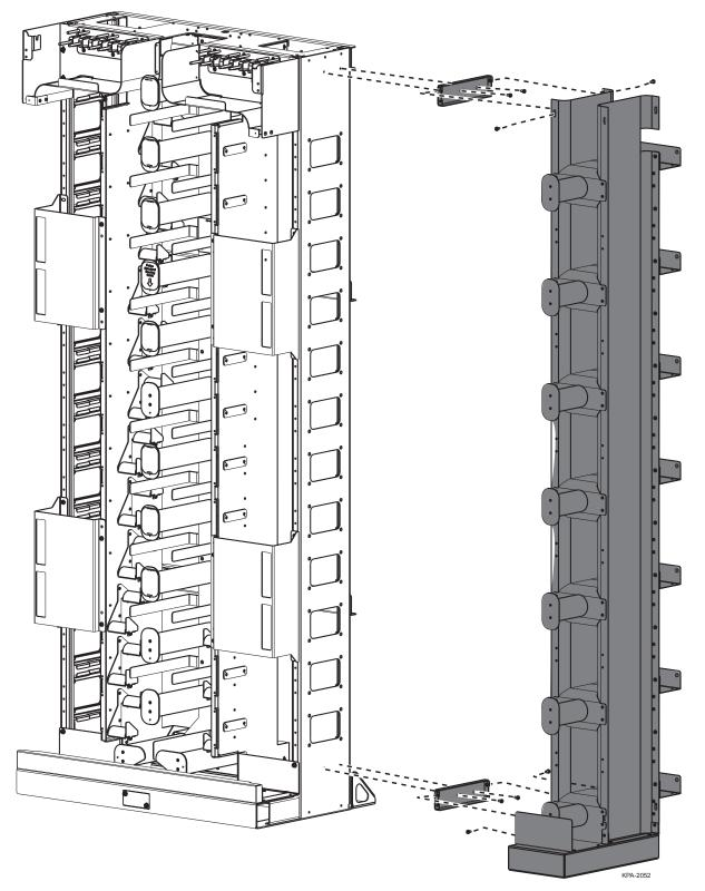
Figure 9 — Installing an IBD
