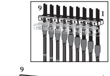
Stagger distance of heatshrink tubing from clamp to provide maximum room for subsequent cable installations. Position first heatshrink tubing approximately 3 inches above the cable guide.
