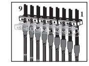
Stagger distance of heatshrink tubing from clamp to provide maximum room for subsequent cable installations. Position first heatshrink tubing approximately 3 inches above the cable guide.
