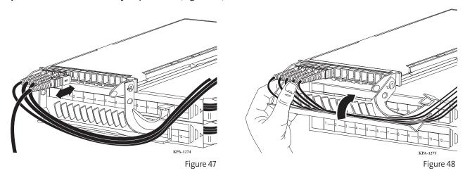
**Step 5:** Push module back into the housing and dress jumper cords in frame as described in Section 11.
