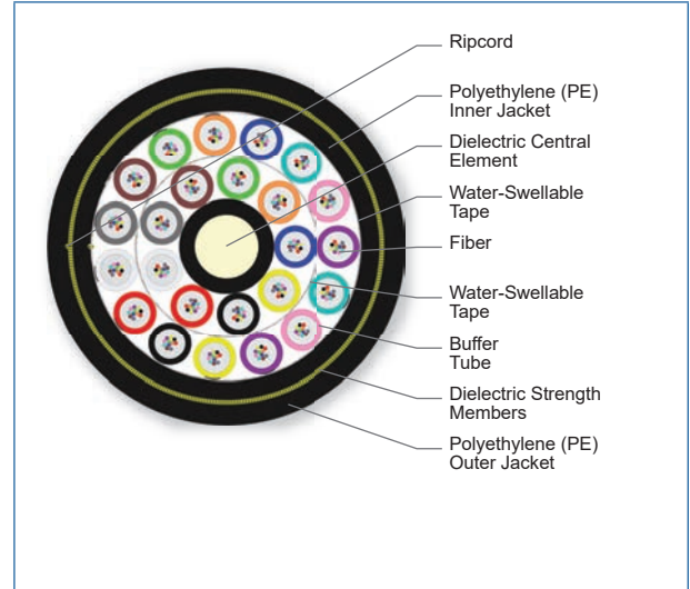
SOLO® ADSS Cable, 288-Fibers
