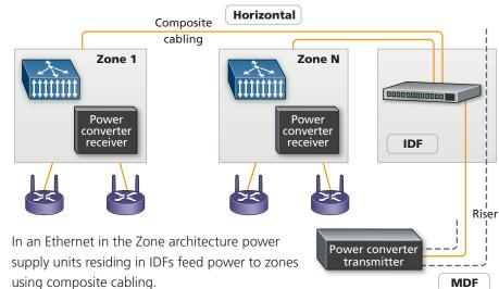
of singlemode fiber with the ability to use larger-gauge copper conductors, we can far exceed the 90-meter limitations of even the best PoE.
