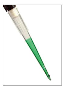
Conventional tip after dispensing 100  $\mu\text{L}$  sample
