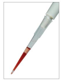
Liquid passes through the conventional filter pipet tips causing cross-contamination.
