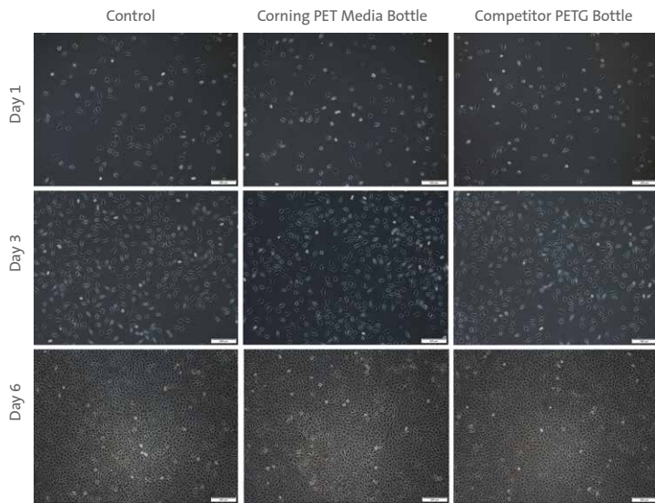
Figure 1. L929 cells cultured with serum that was frozen and stored in Corning PET media bottles or Competitor PETG bottles.
