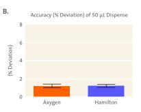
Figure 2. Accuracy (% D) analysis of 50  $\mu$ L tips. The % D of Axygen and Hamilton 50  $\mu$ L tips dispensing (A) 5  $\mu$ L and (B) 50  $\mu$ L using the Microlab STAR liquid handler was determined using the Artel MVS System. There was no significant difference in % D between each brand. Data shown with SD. n = 48.
