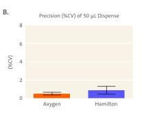
Figure 1. Precision (% CV) analysis of 50 μL tips. The % CV of Axygen and Hamilton 50 μL tips dispensing (A) 5 μL and (B) 50 μL using the Microlab STAR liquid handler was determined using the Artel MVS® System. There was no significant difference in % CV between each brand. Data shown with standard deviation (SD). n = 48.
